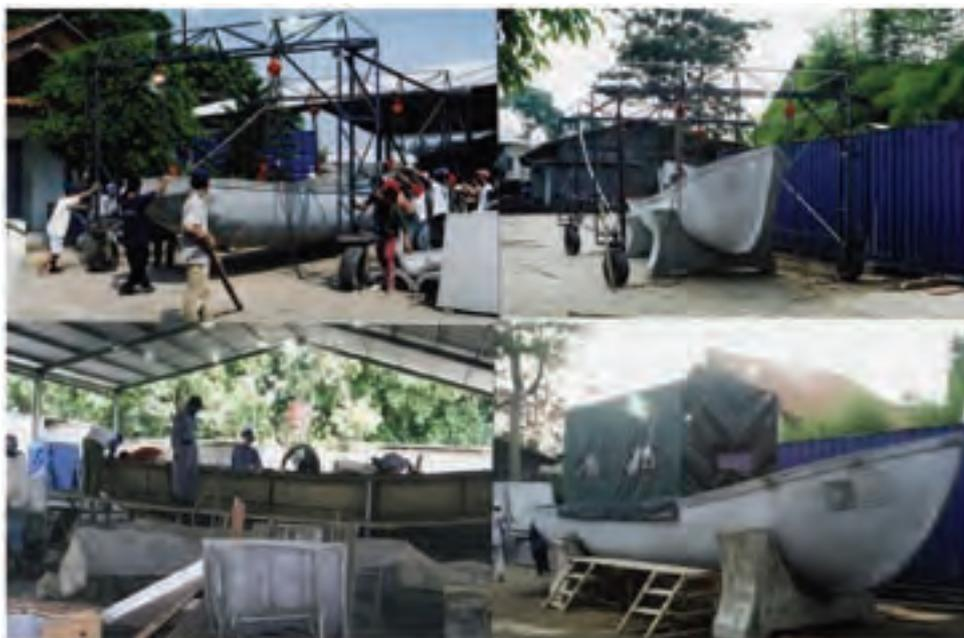
Figure 9 - Manufacture of the third-generation GRC boat
