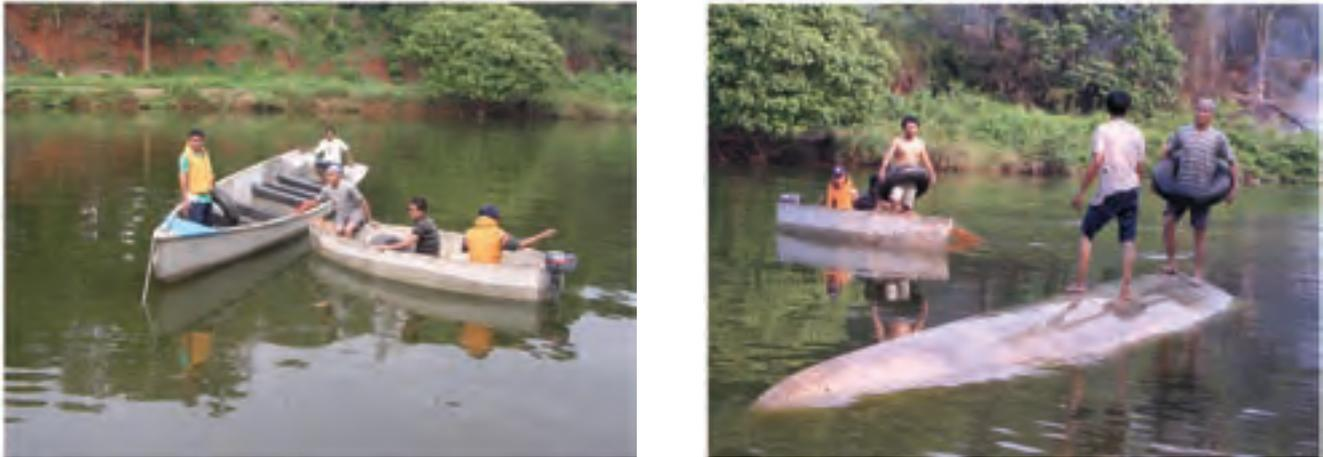
Figure 14 - Capsizing test of the third-generation GRC boat
